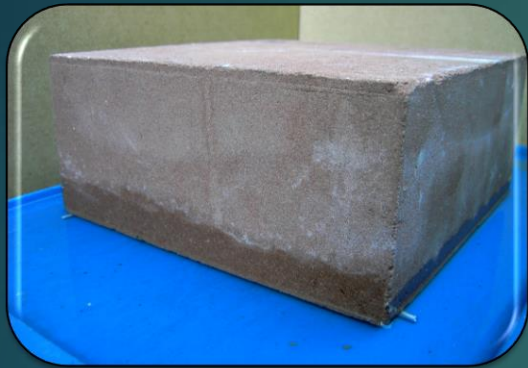
Concrete Water Absorption Test
